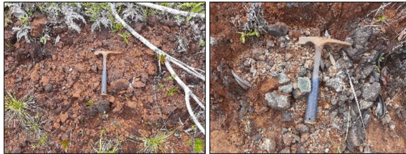
Figure 12. Laterite outcrop (left) and the presence of the mineral garnierite (right) at observation point 42
